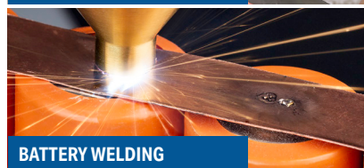
PULSE ARC SEAM WELDING
